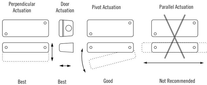
Three configurations are appropriate for interlock applications. The parallel actuation can result in on/off/on signal if the actuator passes by the switch rather than coming to rest in proximity to it. This is NOT a recommended configuration for interlock applications.
